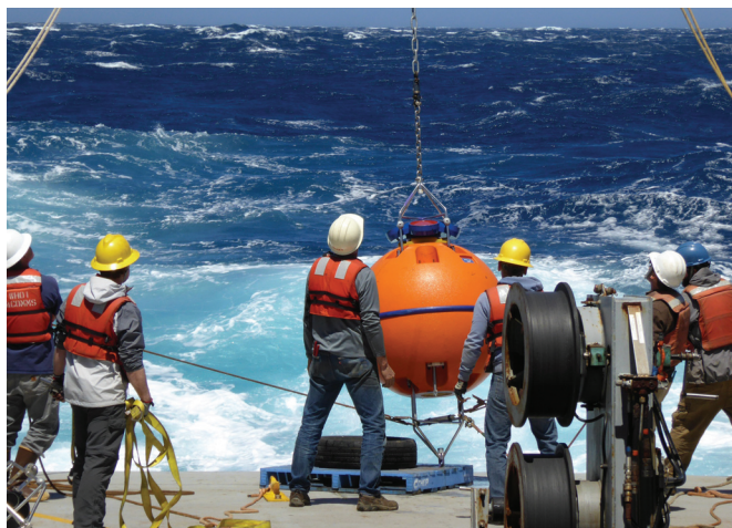
Members of the Tasman Tidal Dissipation Experiment Team recover a DeepWater Buoyancy ADCP buoy aboard the R/V Revelle on an exceptionally windy day in the East Tasman Sea. Photo credit: Sonya Legg, Princeton University.
