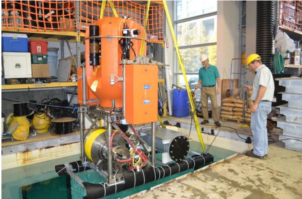
The initial shallow profiler undergoes testing at the University of Washington. DeepWater Buoyancy's syntactic foam systems (in orange) will provide uplift and platform stability for the Regional Scale Nodes portion of the Ocean Observatories Initiative. Photo: Mitch Elend, University of Washington
