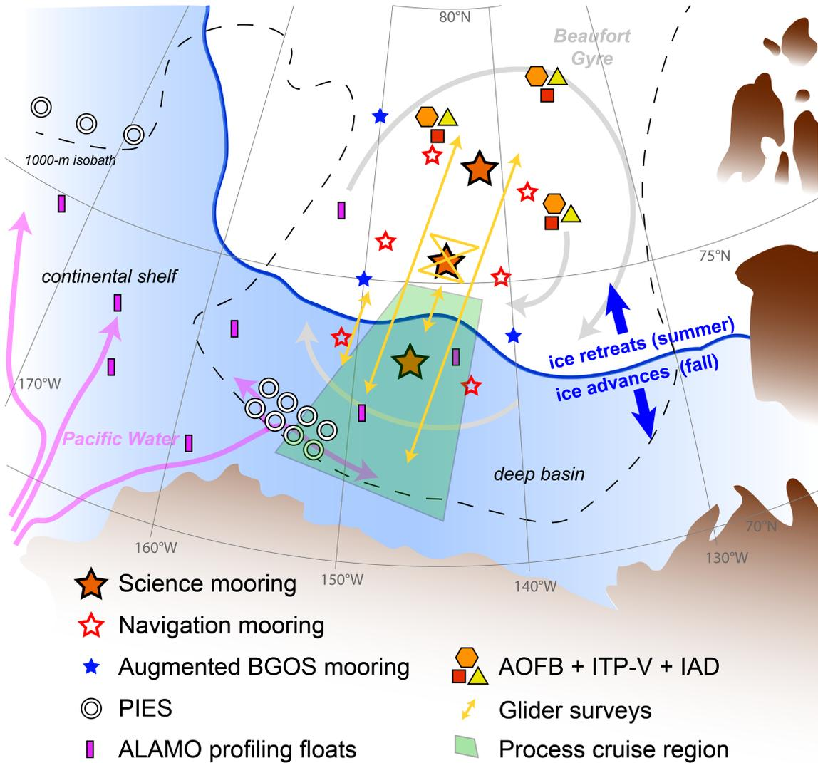
**Figure 6.** Schematic representation of the SODA observing plan. BGOS, Beaufort Gyre Observing System; PIES, Pressure Inverted Echo Sounder; ALAMO, Air-Launched Autonomous Micro Observer; AOFB, Autonomous Ocean Flux Buoy; ITP-V, Ice Tethered Profiler with Velocity; IAD, Integrated Autonomous Drifter.
