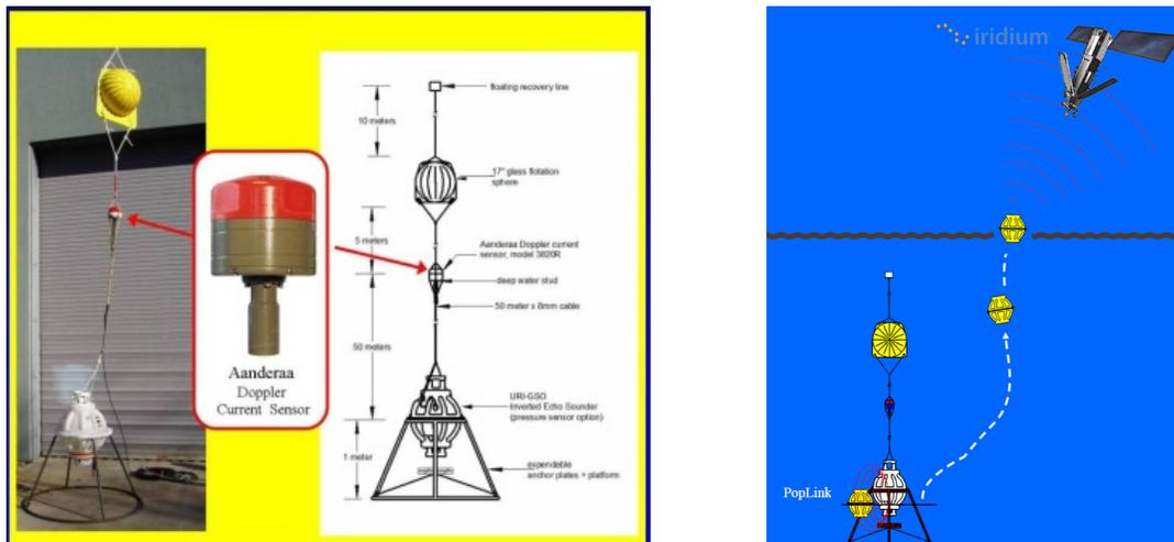
**Figure 8.** (Left) Photograph and schematic of a CPIES. The Pressure Inverted Echo Sounder (PIES) is mounted in a frame and held down by weights through an acoustic release. The current meter is tethered 50 m above the PIES. (Right) A schematic of the PopLink PDS system for yearly transmission of data from a CPIES via Iridium satellite.
