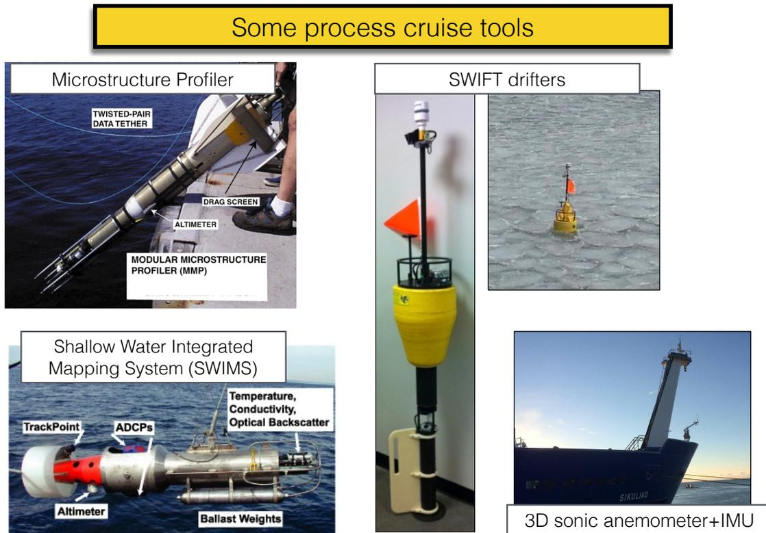
**Figure 10.** Proposed tools to be used during the process cruise. Clockwise from upper left: the Modular Microstructure Profiler (rapid tethered profiling down to 300 m), SWIFT drifters for short deployments from the ship (new versions have ADCPs and C-T chains), meteorological instrumentation on the mast, and the SWIMS towed body.
