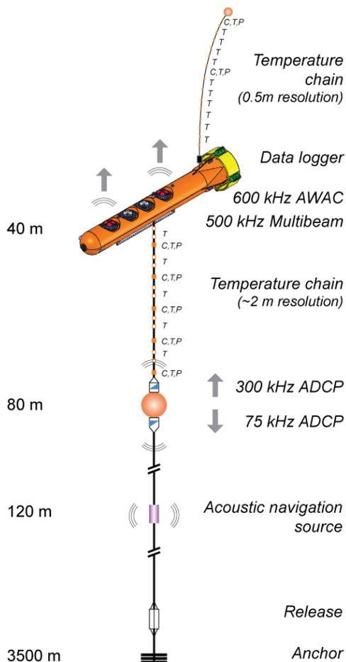
**Figure 9.** SODA-A, B, and C mooring configuration. The upper temperature chain is attached to the Stablemoor float by a weak link. SBE37 MicroCATs and temperature sensors will be deployed to provide coarse resolution below 80-m depth.
